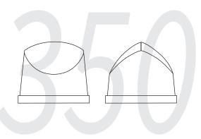
Silicone pads - Series 350 is delivered in hardness 0-30 Shore A, manufactured as standard with wood socket with M6, aluminum or steel socket. We also manufacture customized magnetic click attachment which makes it possible to change pads in seconds without tools or adjustments.
